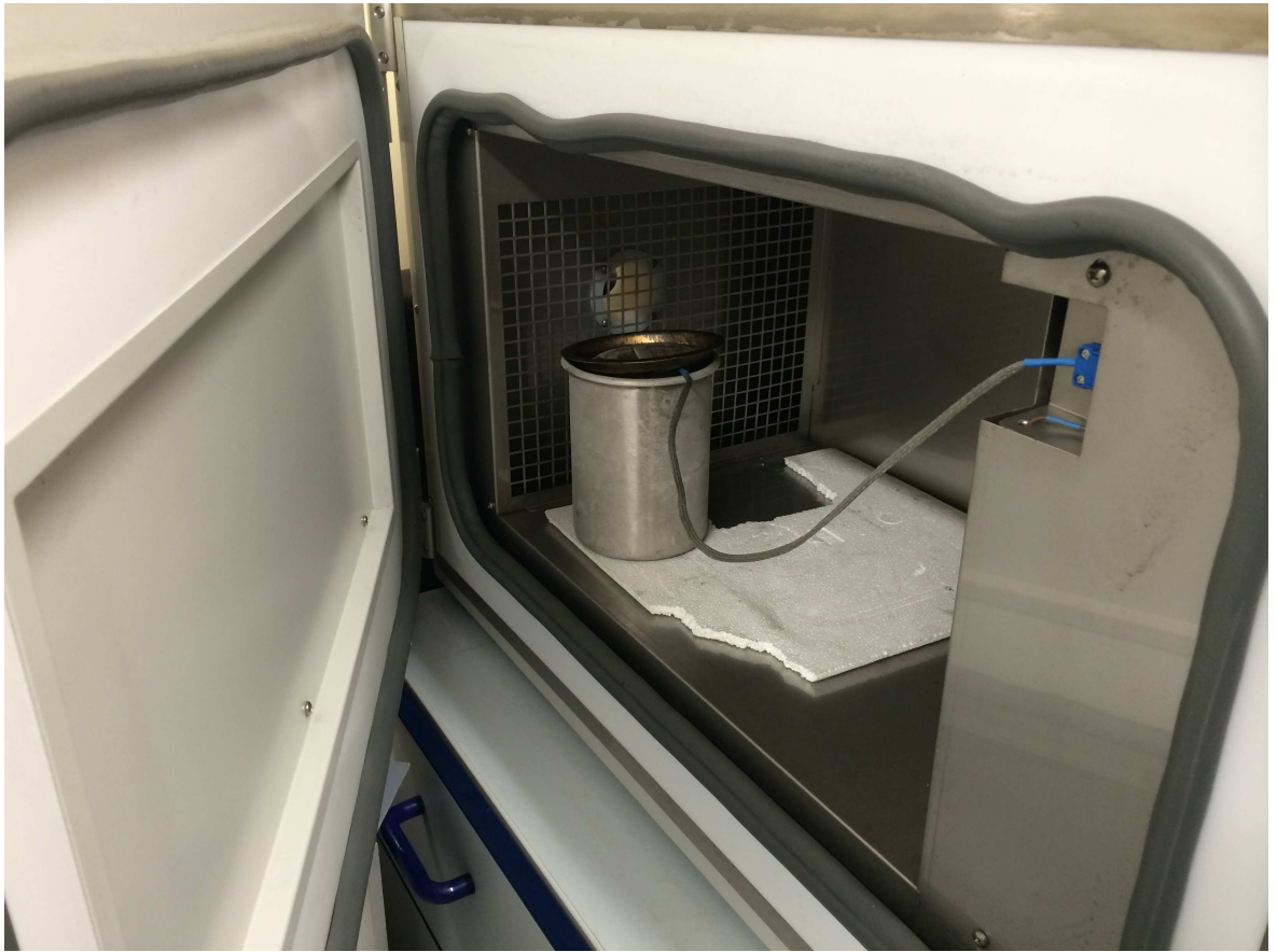
Figure 3.4: The liquid nitrogen freezer in the Impact Lab where the targets were frozen down to -130^{\circ}\text{C} before each shot. Image credit: Taken by author.
