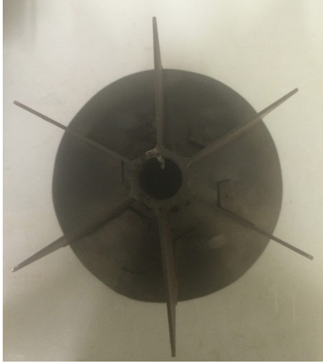
Figure 4.14: The gas diverter is a metallic funnel that is placed in between the target chamber and the gun. Several projectiles hit the back of the funnel leaving traces of damage.
