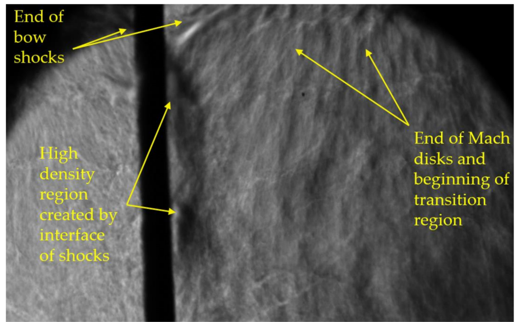
Figure 12. Schlieren of combining air jet ‘curtains’ below the poppet valves, slightly off center of the centrally mounted thermocouple, in the second optical setup, at 5.0 MPa and 1 mm valve lift.
