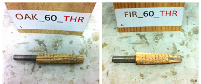
Fig. 14 Wooden parts attached to the hardened resin on the steel bar in the threaded samples in Oak (left) and Douglas Fir (right)
