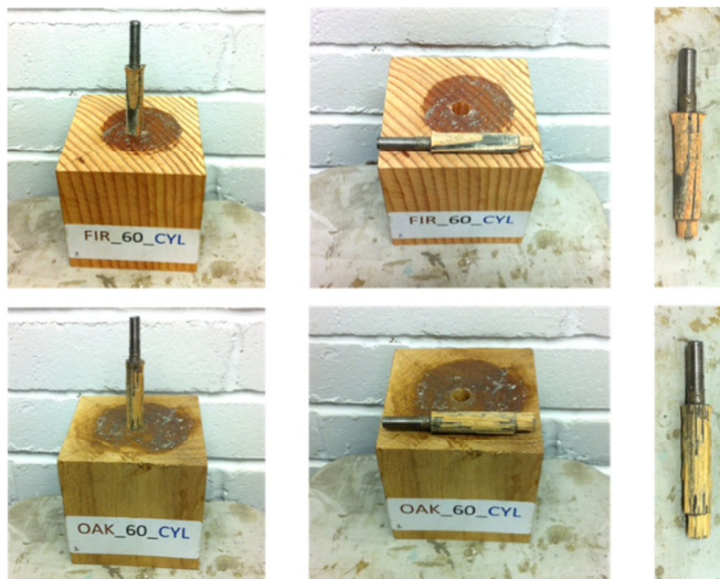
Fig. 12 Failure mode in Oak (bottom) and Douglas Fir (above) samples with smooth and cylindrical borehole after being tested by a pull-out test
