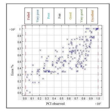
Figure 5-15: Error levels in the pavement classification system for 291 sections.
