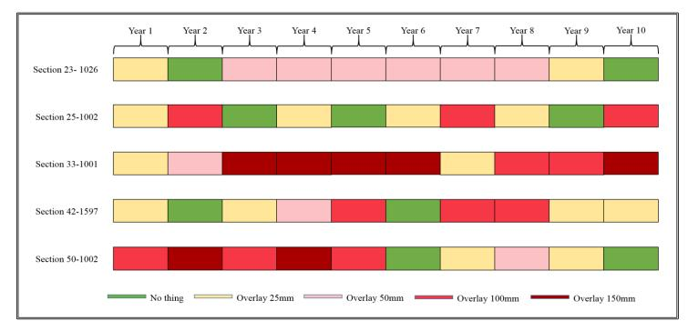
Figure 8-2: Simple presentation of optimal M&R actions plan for five pavement sections.
