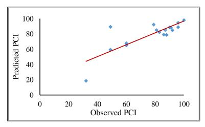
Figure 6-10: Accuracy of the empirical deterioration model for dry non freeze - arterial.
