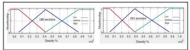
Figure 5-6: Membership functions for Longitudinal and Transverse cracking.
