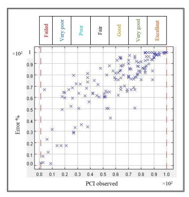
Figure 5-14: Error levels in the pavement classification system for 180 sections.
