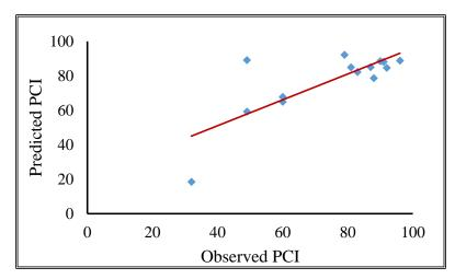
Figure 6-6: Accuracy of the empirical deterioration model for wet non freeze - arterial.
