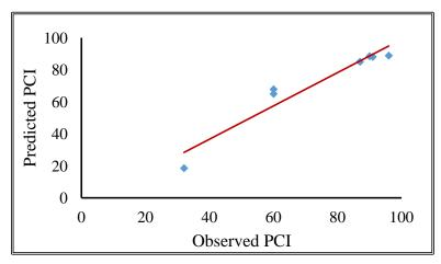
Figure 6-7: Accuracy of the empirical deterioration model for wet non freeze - collector.
