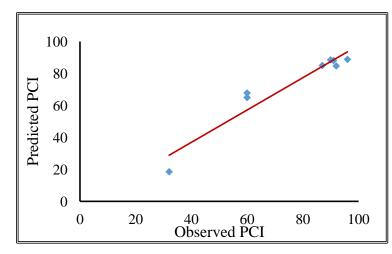
Figure 6-9: Accuracy of the empirical deterioration model for dry freeze - collector.
