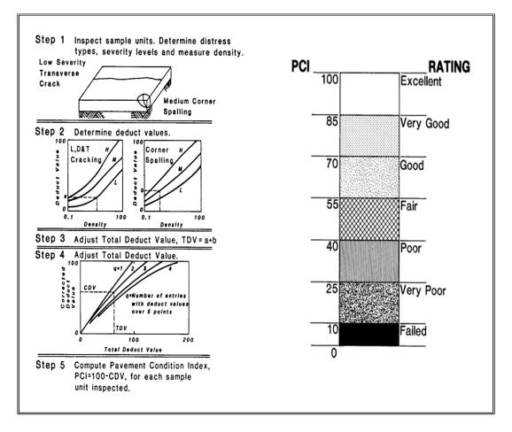
Figure 2-1: Pavement condition index (PCI) calculation procedure (Fwa, 2006).
