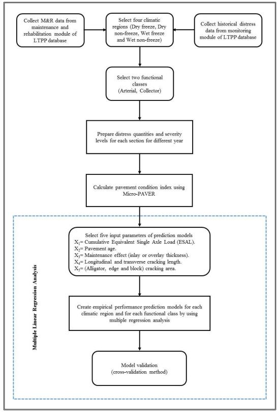
Figure 6-3: Flowchart for a Multi-Input Deterioration Prediction Model (MID-PM).
