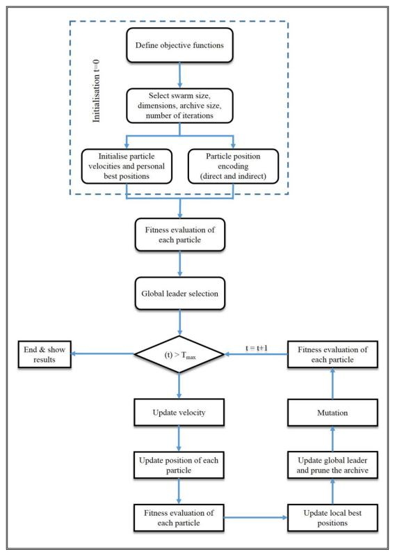
Figure 7-1: Flow chart of the binary barebones particle swarm optimisation algorithm.
