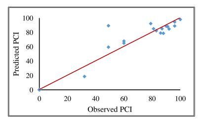
Figure 6-8: Accuracy of the empirical deterioration model for dry freeze - arterial.
