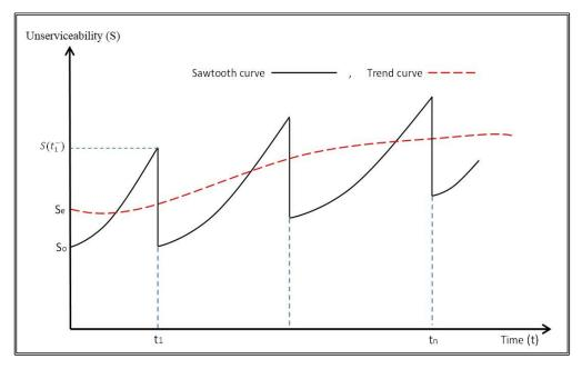
Figure 3-3: Sawtooth curve and trend curve of pavement serviceability (Tsunokawa and Schofer, 1994).
