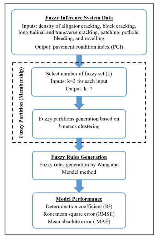
Figure 5-2: Flow chart of a pavement classification model based on FIS.
