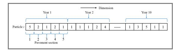
Figure 7-4: Particle position encoding for the pavement maintenance optimisation problem.
