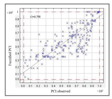
Figure 5-13: The performance of a fuzzy inference system based PCI for 291 sections.
