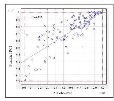
Figure 5-12: The performance of a fuzzy inference system based PCI for 180 sections.
