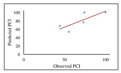
Figure 6-5: Accuracy of the empirical deterioration model for wet freeze - collector.
