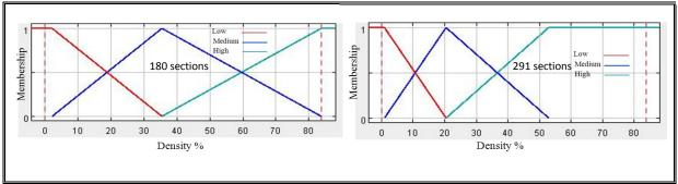
Figure 5-4: Membership functions for Alligator cracking.
