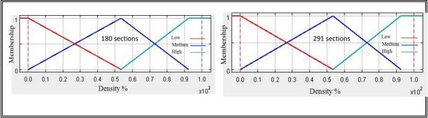
Figure 5-5: Membership functions for Block cracking.
