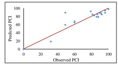
Figure 6-4: Accuracy of the empirical deterioration model for wet freeze - arterial.
