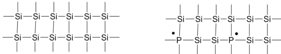
Figure 17. Silicon 2D lattice and phosphorus-doped silicon 2D lattice.
