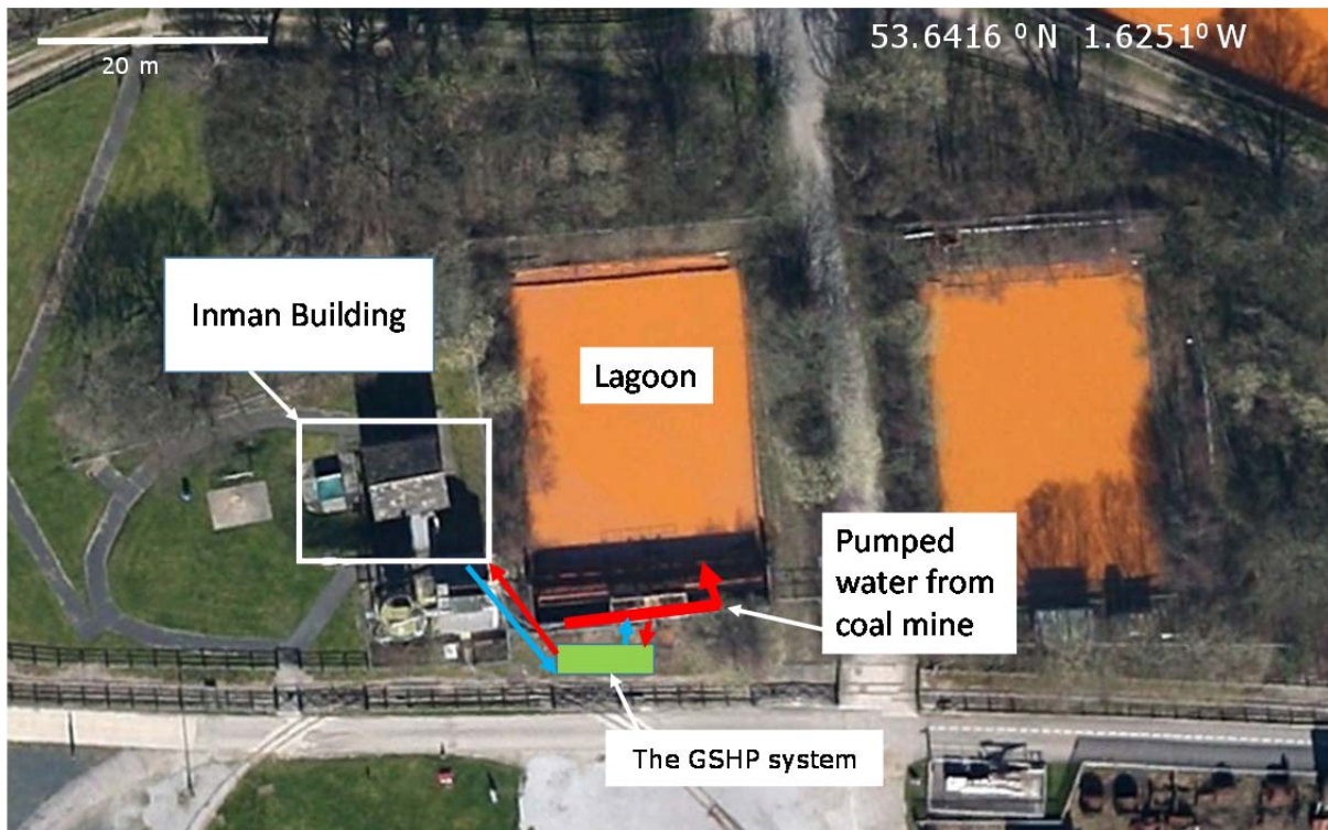
Figure 2: A Google Satellite image of the location with a schematic diagram of the implementation of the system.
