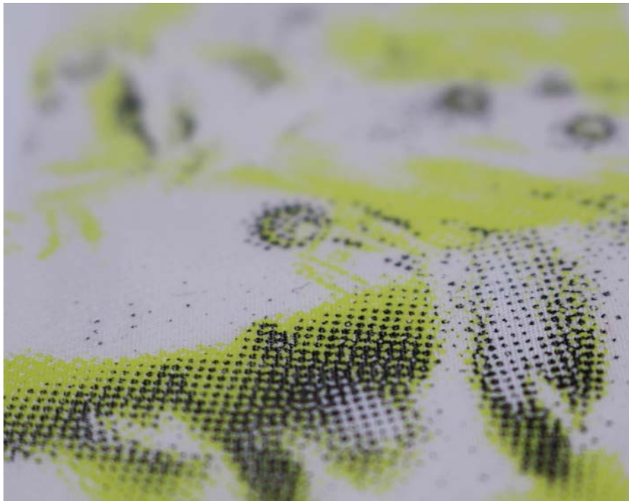
6a: Printed surface before UV exposure
