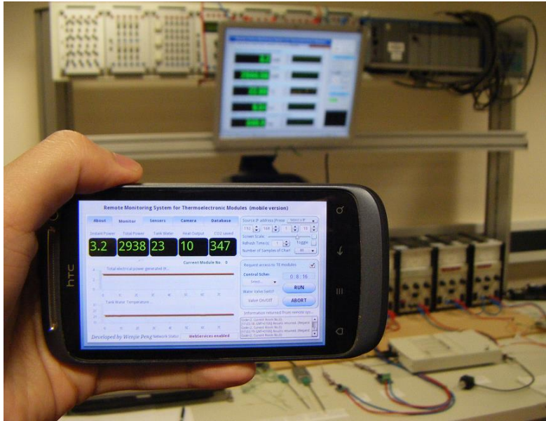
Figure 11 Remote acquisition of working condition data from the primary panel of the server using HTC mobile phone
