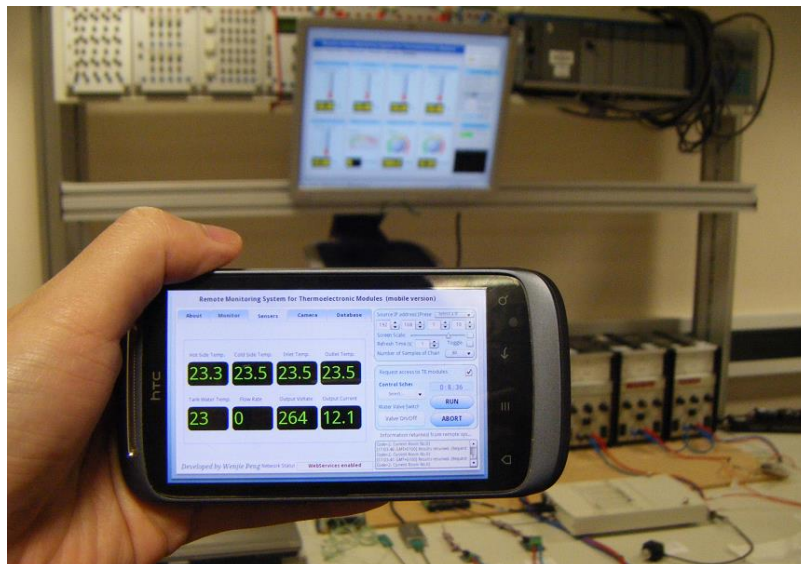
Figure 12 Remote acquisition of working condition data from the secondary panel of the server using HTC mobile phone
