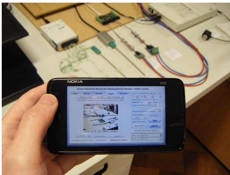
Figure 10 Real-time display of the video which monitors the operation of TEGs using Nokia mobile phone
