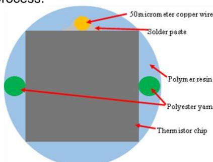
Fig. 3: Cross sectional view of the Micro-pod
