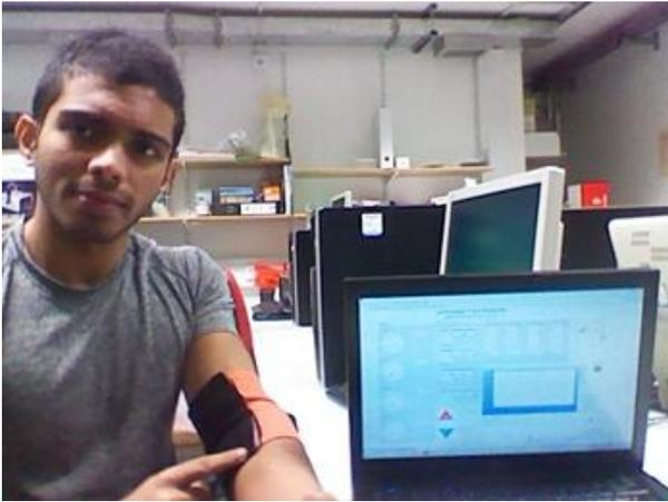
Fig. 5: Armband knitted using the ETS yarn
