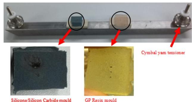
Fig. 2: Soldering Jig designed for forming interconnects
