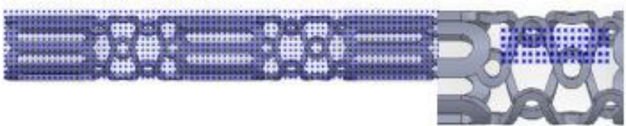
Figure 2: coating patterns of Cypher® stents a) for large areas of the stent struts, b) for smaller areas with thin struts
