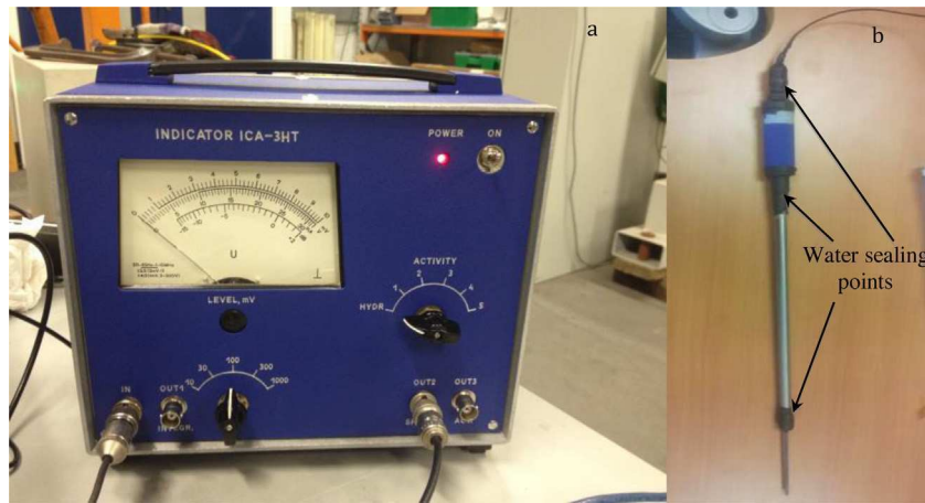
Fig. 1. A cavitometer device (a) ICA-3HT electronic unit and (b) a high-temperature hydrophone connected to the unit (the hydrophone is sealed for calibration in water).
