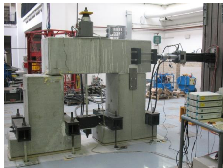
Figure 2. Experimental setup of a monotonic shear test on a beam-to-column dowel connection
