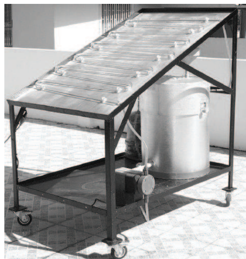
FIGURE 3: Photograph of solar photochemical reactor installed and in operation, North-East, Trinidad, West Indies.
