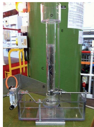
Scheme 1 SANS sample environment for studying foams.
