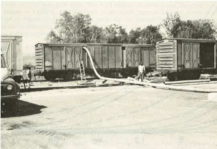
Fig. 7. Filling a railtruck with grain in bulk. Double-ply cardboard sheeting contains the grain during filling, allows the temporary insertion of pneumatic conveyor tubing, and facilitates the sealing and closure of the doors immediately after the introduction of fumigant.
