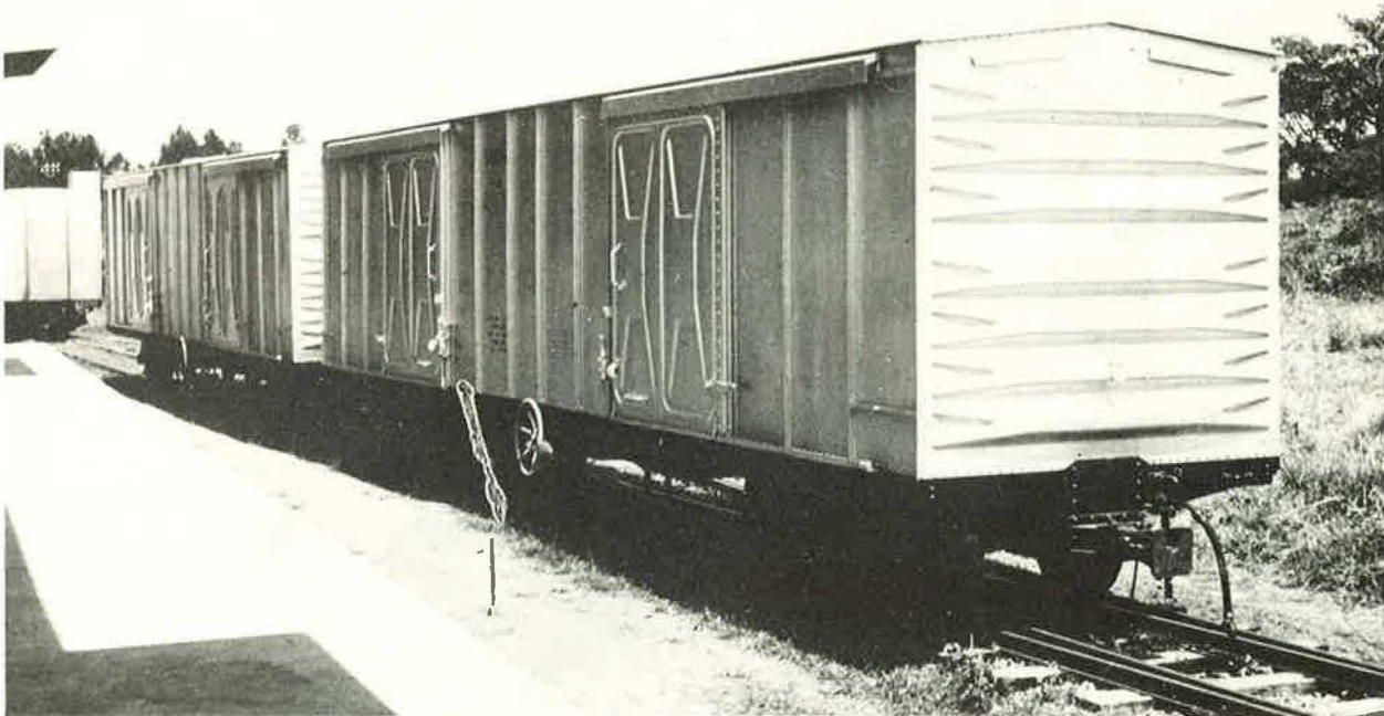
Fig. 2. Railtrucks of more recent design which can be sealed effectively and which retain fumigant reasonably well.
