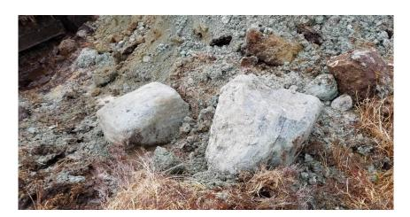
**Figure 7.** Two of the ten boulders found within the excavated volume are shown. Their diameters are approximately 0.4 m and 0.6 m, and they were distributed throughout the 633 m<sup>3</sup> of the 2019 excavation, but similar boulders were not observed on the surface of the peat bog.
