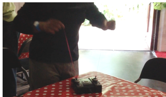
Figure 1: A workshop participant plays a digital instrument built with the Gametrak controller, which senses 3D position of the user's hands using two strings.
