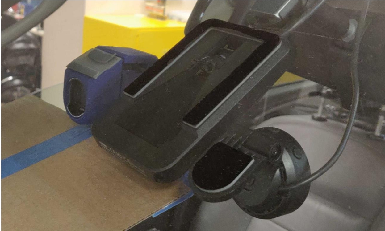
Figure 15: Vision Setup; Mobileye 6 (Center) and Diagnostic Camera (Left)
