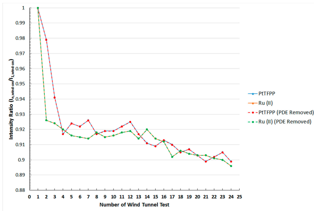
Figure 12. Relation between the normalized intensity ratio and the number of wind tunnel test for the PtTFPP and Ru (II) polymer-based pressure-sensitive paints.
