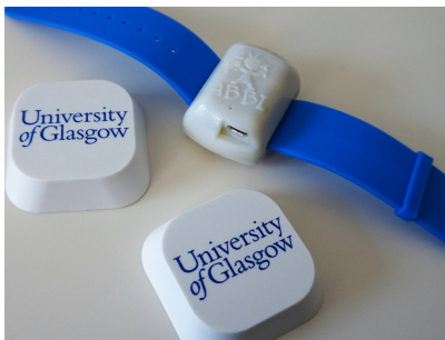
Figure 1: ABBI bracelet prototype and two of the kontakt.io iBeacons used by our system. Future iterations of the bracelet will have a smaller and more appealing design for children.
