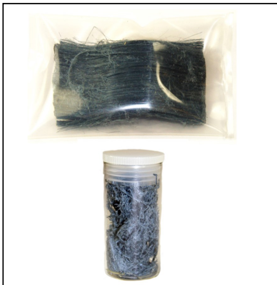
Fig. 5. Crocidolite, also known as blue asbestos, is a variety of the amphibole riebeckite. (top: OUMNH-Min16130, specimen c.60 x 32mm; bottom: OUMNH-Min26175 from Australia, 53mm high tube).
