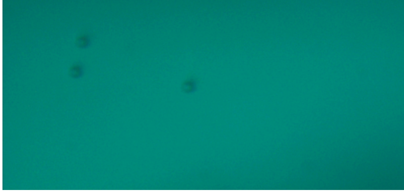
Fig 1: Polystyrene beads flowing in a capillary tube; this is a single frame from the input video. We will use it to illustrate background subtraction and morphological operations.
