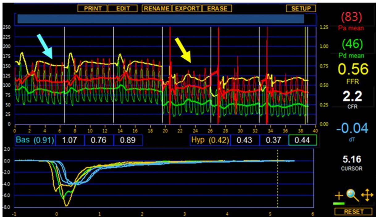
Fig. 1. A hemodynamic recording obtained from a diagnostic pressure- and temperature-sensitive guidewire (PressureWire Certus™, St. Jude Medical, Mn.) located in a culprit coronary artery at the end of primary PCI. The blue arrow represents the thermomodulation recordings during resting conditions before adenosine administration. The thermomodulation curve represents the transit time for the change in temperature detected by the distal guidewire thermistor following intra-coronary bolus injection of saline (room temperature) via the guiding catheter. The subsequent yellow arrow represents the transit times for thermomodulation curves following intra-coronary injections of saline during hyperemia with adenosine (140 µg/kg/min). During hyperemia, there is evidence of a reduction in arterial blood pressure depicted by the yellow arrow, reflecting the typical hemodynamic response in the systemic and coronary circulations to intravenous adenosine. Hemodynamic recordings were assessed with vendor software (RADView Version 2.2, St. Jude Medical, Mn.). The systolic blood pressure and diastolic pressure during at least 3 cardiac cycles in steady-state conditions at rest and during hyperemia were assessed. (For interpretation of the references to color in this figure legend, the reader is referred to the web version of this article.)
