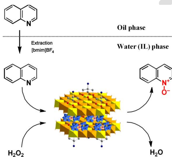
Fig 9. The proposed mechanism for the denitrogenation of the oil phase and consequent catalytic oxidation of 4-picoline in the aqueous phase by Tris-LDH-La(PW 11 ) 2 in the presence of H 2 O 2 .
