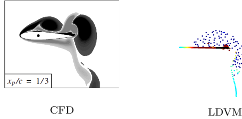
Figure 13: Vorticity plot from CFD (Kinsey & Dumas [26], reproduced with permission) for t/T = 1.0 compared with flowfield from LDVM for t/T = 1.0 .
