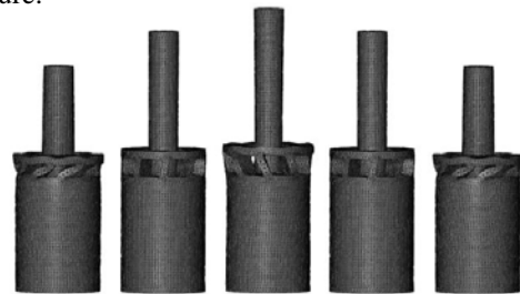
FIGURE 3. A half-cycle of simulated behavior in the smart horn at 20 kHz.
