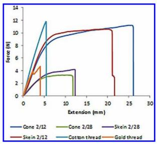
Figure 12 Force vs. elongation of cotton and wool yarns.
