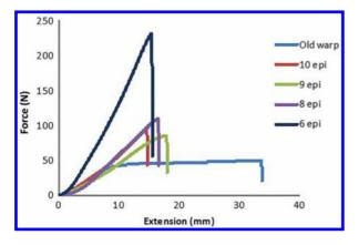
Figure 11 Force vs. elongation of the warp yarns.
