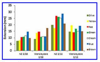
Figure 4 Maximum extension of the wools at break point.
