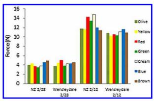
Figure 6 Maximum tenacity at sample failure point of the wools.
