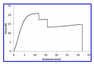
Figure 8 Graph of force vs. extension, of the compound yarns, two 2/28 and one 2/12.
