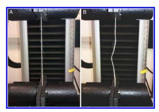
Figure 3 (A) Wool strand before application of force; (B) force released after stretching wool beyond elastic point.
