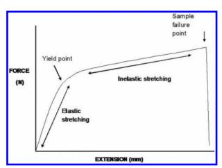
Figure 2 Force vs. elongation curve for wool.
