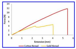
Figure 9 Graph showing force vs. extension for cotton and gold-coated threads.
