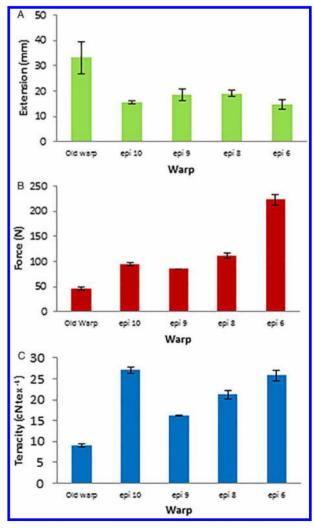
Figure 10 (A) Maximum extension at break; (B) maximum force at break; (C) maximum tenacity at break.
