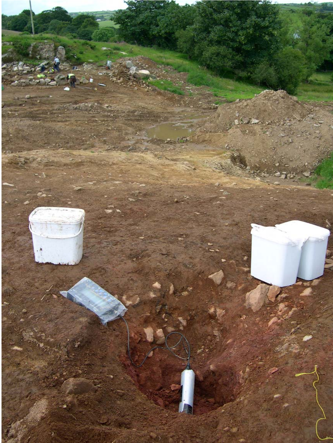
Figure 3.4. Newry Ring Fort Pit 1 (NW quarter of site complex within ring ditch). Illustrating pit location, shape, fill and cover sediments, and arrangement of gamma spectrometry measurement.
