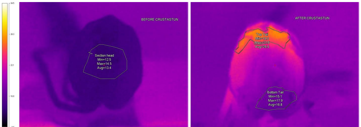
Figure 5. Thermal images taken through a transverse section of the cephalothorax (“head”) A) before and B) after being subjected to a standard Crustastun procedure. Values refer to the outlined areas.
