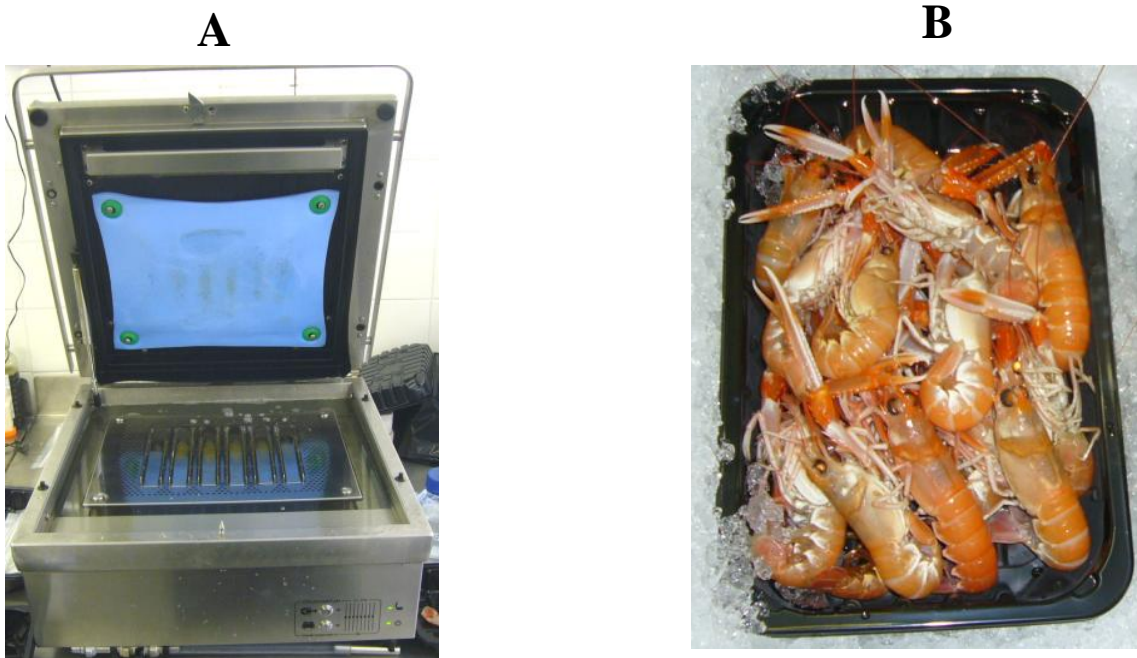
Figure 1. A. The Crustastun Prototype I. B. Langoustines on ice after being electrocuted in the Crustastun.
