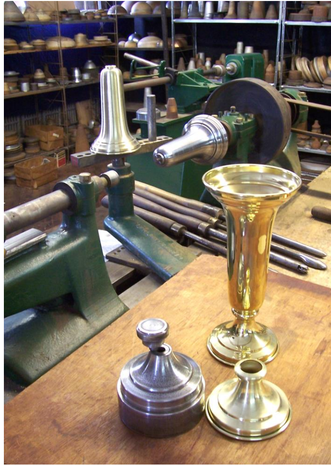
Figure 1-2 - Some bespoke spun parts and the mandrels used to make them (Photograph by Terry Tynan licensed under CC BY-SA 3.0)
