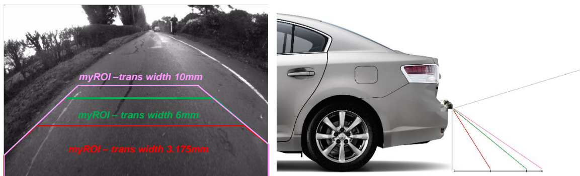
Figure 4. Left- Depiction of myROI on top of a video frame captured by a parking camera (trans holds for transverse); a transverse crack with 3.175mm width can be found within the red shape, a transverse crack with 6mm width can be found within the green shape and one with 1cm can be found within the magenta shape, Right- Depiction of extension of myROI at the back of a vehicle
