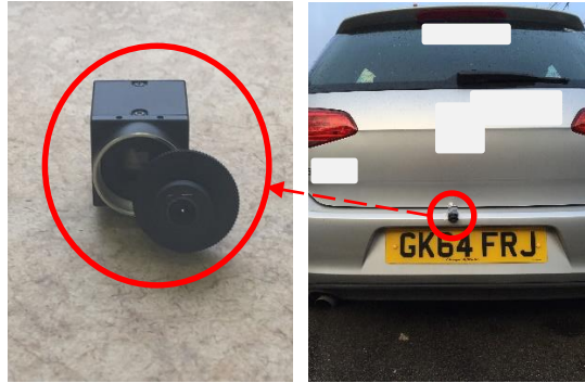
Figure 3. Left - Hardware used for the calculation of myROI; Right - The position of the camera at the rear of a vehicle
