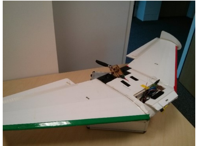
Figure 1: The delta-wing airframe with two-channel elevon control.
