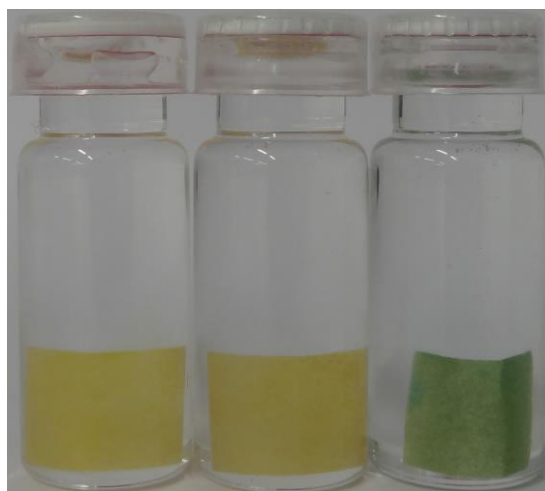
Figure 7. Samples of Ethaline (left) Glyceline (middle) and Reline (right) with 20 wt% water and each containing a sample of universal indicator paper.
