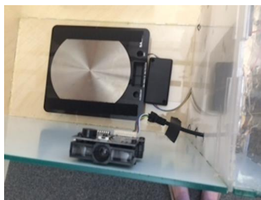
Figure 2: The barcode scanner and weighing scale mounted inside the Beautybox, with the weighing platter removed and the cables threaded through apertures in the instrument panel.
