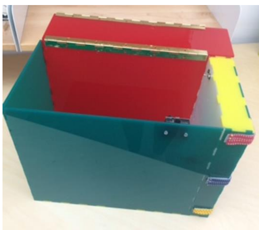
Figure 1: The Beautybox with open lid, showing the barcode scanner mounted on the front, and the assembly compartment on the right.
