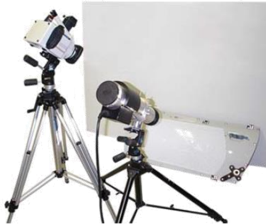
797 Figure 1: Projector and camera setup for extracting absolute measurements in manufacturing 798 industry (Ganci and Brown, 2008)
