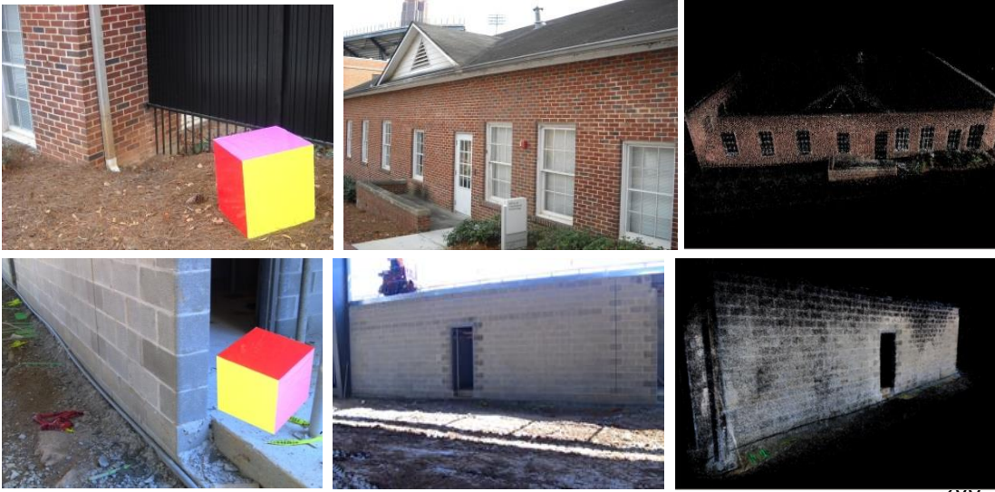
969 Figure 14: Samples of the generated PCD for outdoor settings: Campus building (top) and 970 construction wall (bottom)
