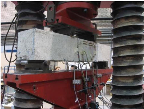
Figure 8: Setting of the four-point bending test (1-A)
