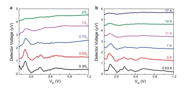
Figure 3: Influence of QPC conductance and temperature on the operation of spin FETs. a, Detector voltage as a function of  $V_{\rm M}$  at various  $G_{\rm QPC}$  values, ranging from  $0.3G_0$  to  $2G_0$ , while T is fixed at 0.03 K. Data are vertically offset by 1  $\mu{\rm V}$  for clarity. b, Same as a for various temperatures ranging from 0.03 to 17 K, for  $G_{\rm QPC}=0.3G_0$ .
