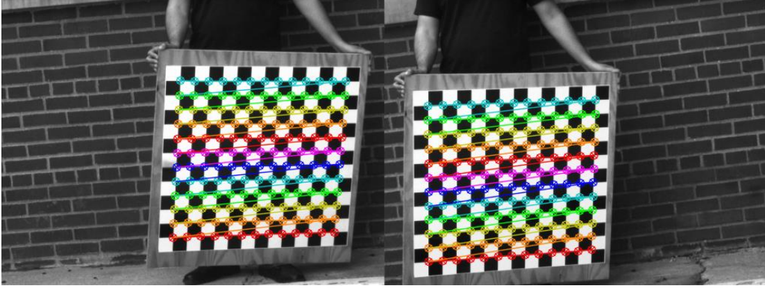
Figure 4: Automatically detected and matched calibration board corners
