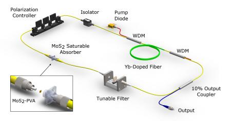
Fig. 3. Q-Switched fiber laser cavity schematic.
