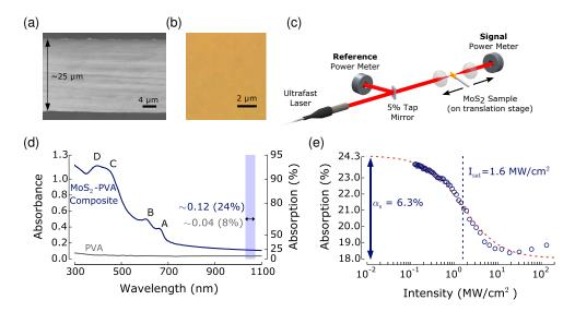
Fig. 2. Characterization of the MoS<sub>2</sub>-polymer SA film. (a) SEM of the cross-section and (b) optical micrograph confirming the absence of aggregates. (c) Z-scan setup. (d) Optical absorption of the film, with the highlighted region indicating the range of operation of the tunable Q-switched laser. (e) Nonlinear absorption profile showing saturable absorption.
