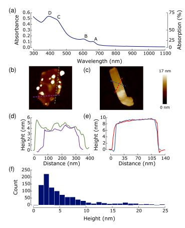
Fig. 1. Characterization of the dispersed  $MoS_2$  flakes. (a) Optical absorption of dispersed  $MoS_2$ . (b-f) Characterization via AFM: (b-e) images of typical flakes and flake thickness profiles, (f) distribution of flake thicknesses.
