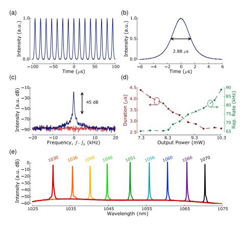
Fig. 4. Q-switched laser characteristics: (a) Pulse train. (b) Single pulse profile. (c) RF spectrum of fundamental frequency,  $f_0$ =74 kHz. (d) Variation of repetition frequency and pulse duration with output power. (e) Output spectra for Q-Switched operation at various wavelengths. The wavelength could be continuously tuned between 1030 and 1070 nm using the tunable filter.
