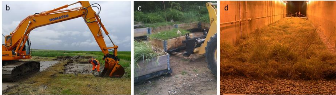
285 Figure 1 | Experimental set-up and photographs of excavation. a , General experimental set-up in 286 the wave flume, with position of recording equipment relevant to reported results. b , Excavation of 287 marsh blocks, northern German Wadden Sea (53°42.754 N, 07°52.963 E). c , Marsh blocks with 288 Elymus vegetation cover prior to positioning in the flume test section. d , Reassembled salt marsh 289 inside the 5-m-wide flume, looking towards the wave generator; lamps are mounted at about 3m 290 above the soil surface.
