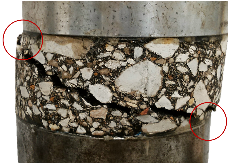
Fig.9 Diagonal shear failure plane of an asphalt concrete in octahedral shear strength tests
