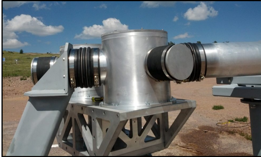
Figure 5: Telescope beam relay can with mirrors installed. This can and its associated optics are under long-term stability testing outside the beam combining facility at MROI.
