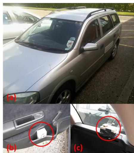
Fig. 4. (a) Car; (b) Transmitting node located in the passenger side rear door; (c) Receiving node located in the boot on the driver side.
