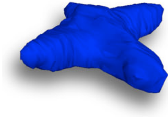
Fig. 5 Three dimensional representation of diffuse scattering profile associated with a tweed microstructure in a superconducting oxide sample in Fig. 2 (reanalyzed after Locherer et al. 1996).
