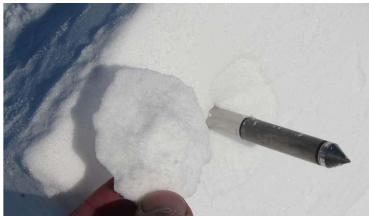
Figure 4.14: During unconfined penetration a chip of snow fractures from the side of a block.
