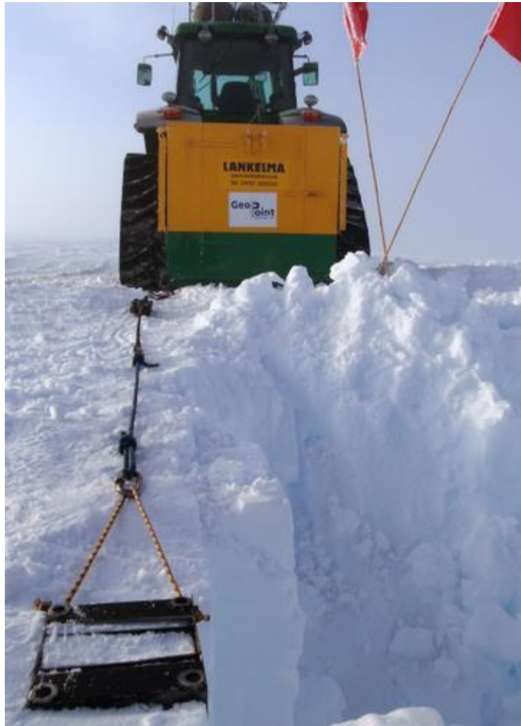
Figure 3.14: Typical shear test set-up shows tractor about to load shear frame inserted into surface snow layer, adjacent to snow pit #1.
