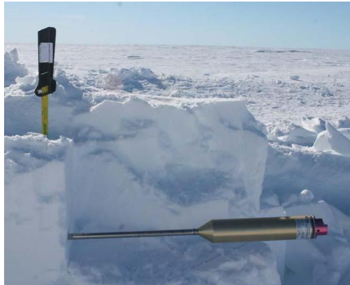
Figure 4.10: Horizontal method of testing for compacted zone ahead of cone.
