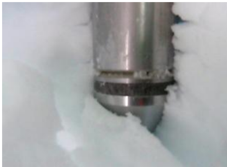
Figure 5.21: Screen shot of a 36.7 mm diameter standard cone slowly advancing in cut-away hole.
