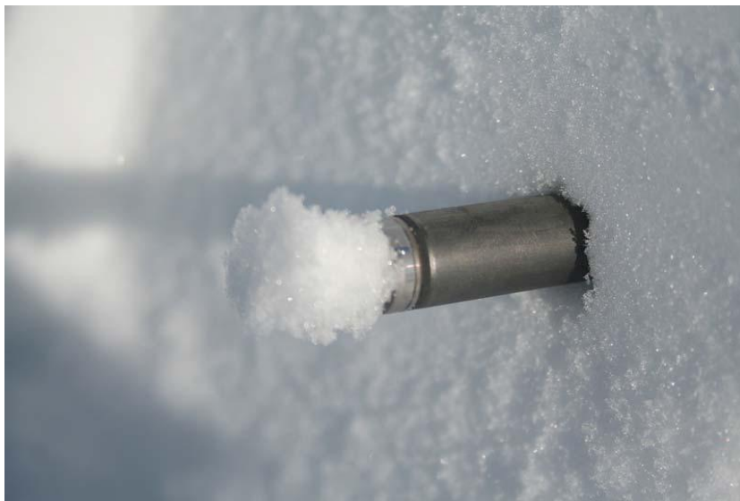
Figure 4.12: A plug of snow was observed to form ahead of the cone upon exit from block of snow.
