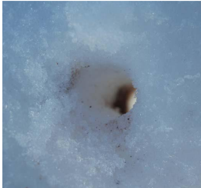
Figure 4.13: Chilli flakes sprinkled onto the snow prior to penetration are shown to have been pressed into the hole sides (dark band) during cone penetration; no flakes were observed in snow ejected ahead of the cone.
