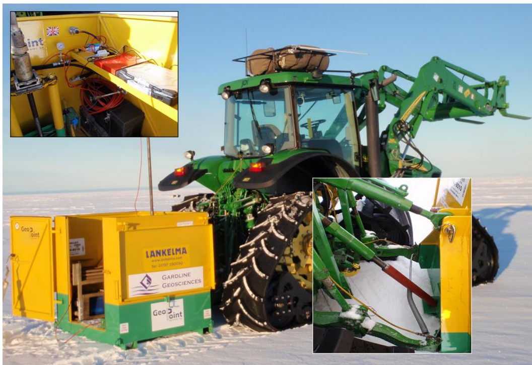
Figure 3.8: UK11 configured and fitted for CPT. Insets show rigid link installed and data collection equipment.
