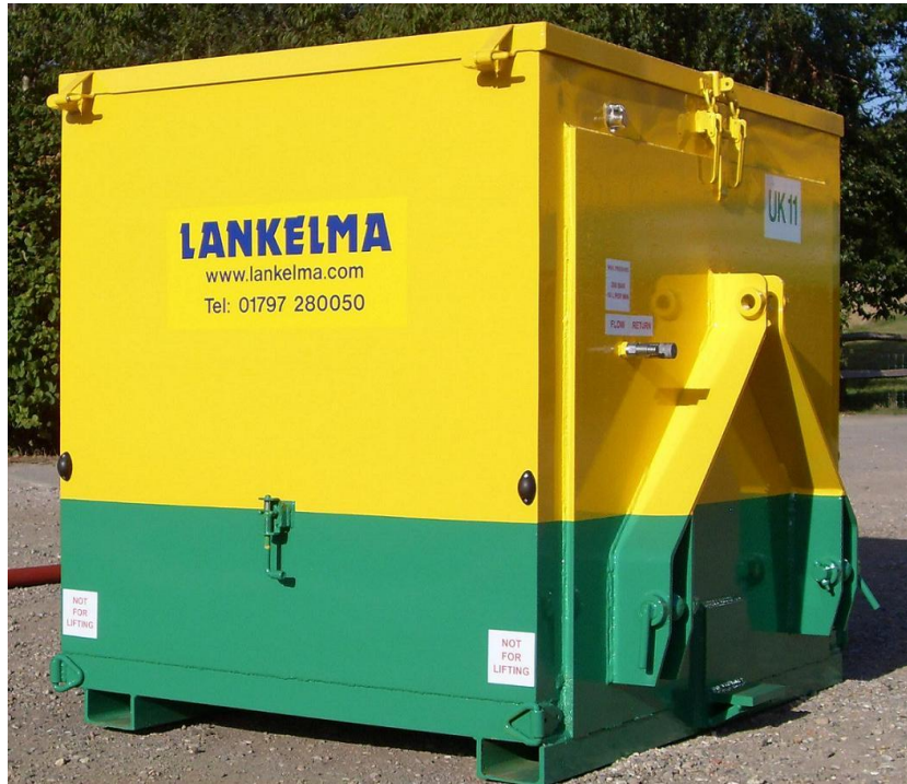
Figure 3.6: ‘UK11’ constructed by Lankelma within which CPT equipment was mounted. Note mounting points for tractor 3-point linkage and input ports for 12V electrical power and hydraulics.
