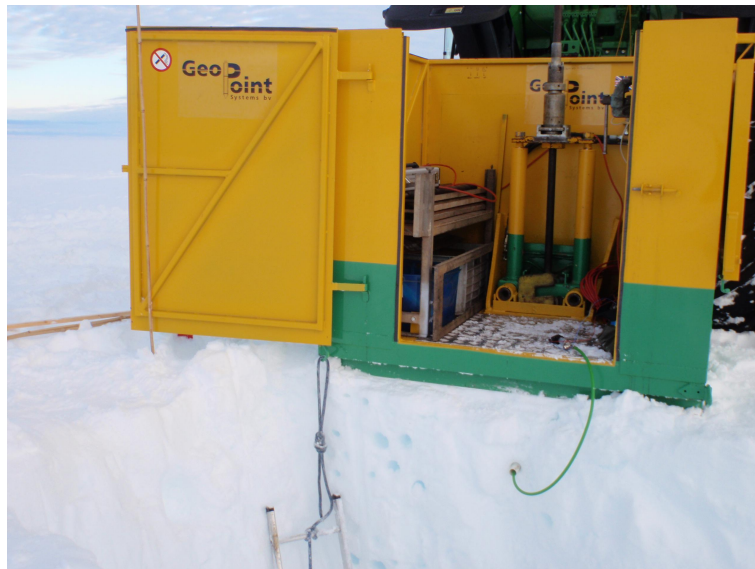
Figure 3.19: Setup for investigating pressure-bulb beneath cone or flat plate. The rubber pipette-bulb was inserted into the snow in a location estimated to be directly beneath the path of the cone before CPT was then conducted.
