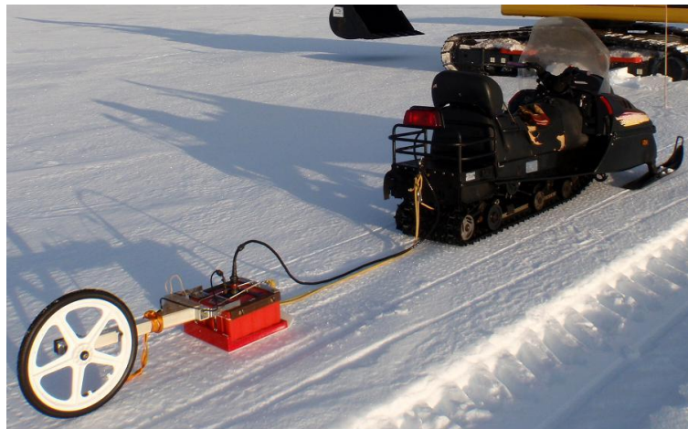
Figure 3.20: The GPR was towed behind a skidoo and operated in ‘distance’ mode.
