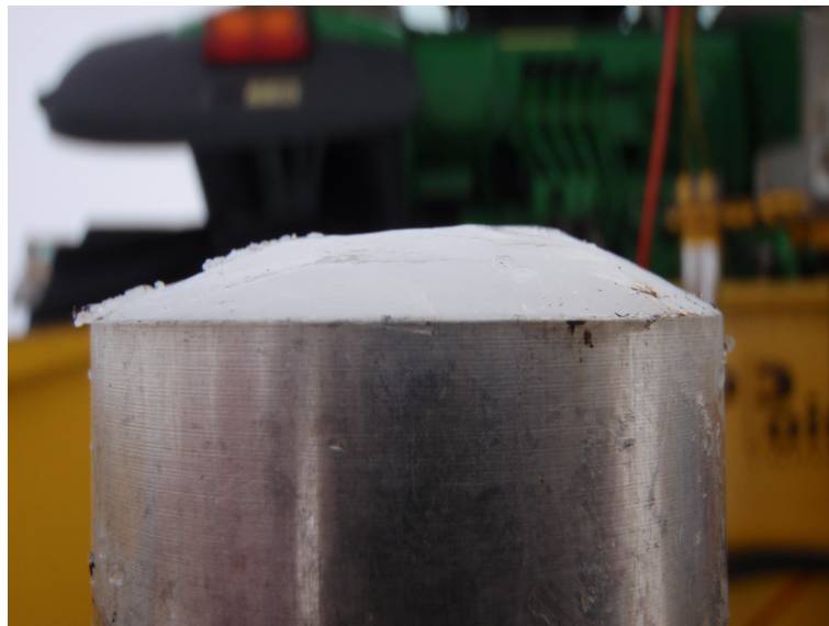
Figure 5.24: Low-angle conical plug routinely observed on flat-plate post-test.
