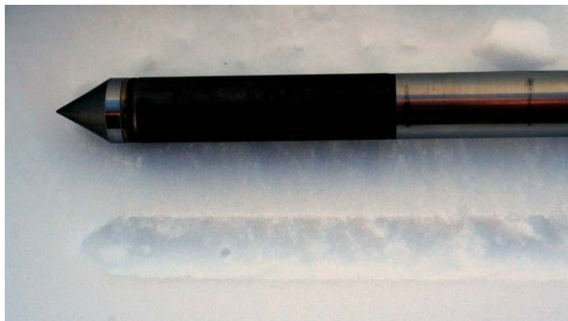
Figure 4.11: Comparison of the penetrometer with the cavity formed from penetration shows no visible evidence of a compacted zone of snow ahead of the penetrometer.
