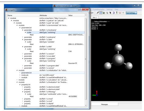
Figure 3 A compchem-compliant document read into the Avogadro [39] browser and computational chemistry manager. The structure of the document is shown with the primary subdivisions. Each piece of information is in a precisely specified position in the hierarchy, so that it may easily be discovered by processing software. For example the hostname must occur as a scalar child of parameter with a specific @dictRef. and so on.
