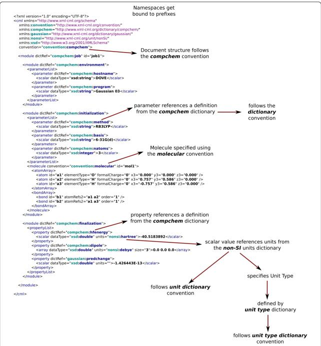
**Figure 1** The primary semantic components of CML. Elements in a document link to conventions, dictionaries and units through attributes. The referenced resources are themselves constrained by specification documents (convention spec, dictionary spec, system of units) with unique URIs. Within the dictionaries and the unit collections, every entry has a unique ID and when combined with the dictionary URI produces a globally-unique identifier.
