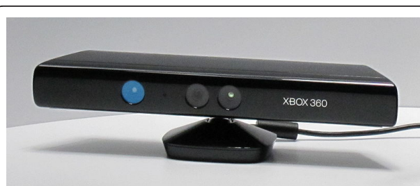
Figure 10 The Microsoft Kinect. This connects to a computer via a USB connector, making it a powerful way to communicate with computers. The infrared transmitter is on the left.
