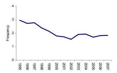
Figure.8 kWh-distibuted weighted average CAIDI over time
