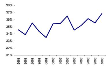
Figure.6 kWh-distributed weighted average SAIDI over time
