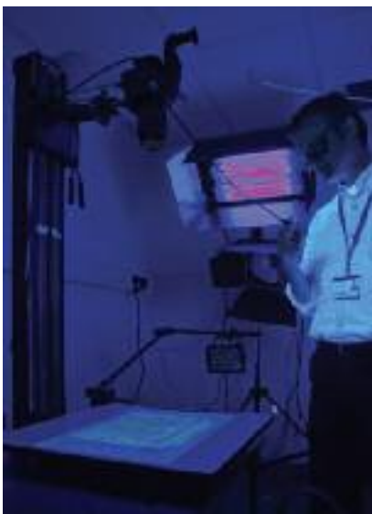
A palimpsest being imaged using ultraviolet light.
