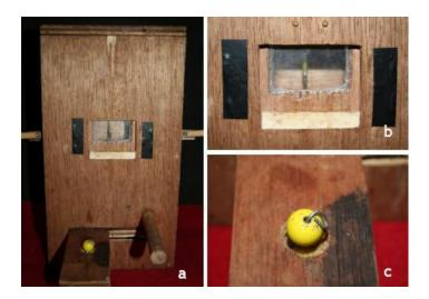
**Figure 32.** The test apparatus (a) and detailed pictures of the feeder opening (b) and the yellow wooden ball (c).
