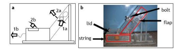
**Figure 41.** A diagram (a) and photograph (b) of the test apparatus. (a): Letters and arrows indicate the two different actions on each of the two parts of the apparatus; numbers represent demonstrators 1 and 2. The circle shows where the Kinder egg was placed at the beginning of each trial. (b): Bold red lines show the two parts of the apparatus: vertical and horizontal. Arrows point at the release mechanisms that had to be manipulated.
